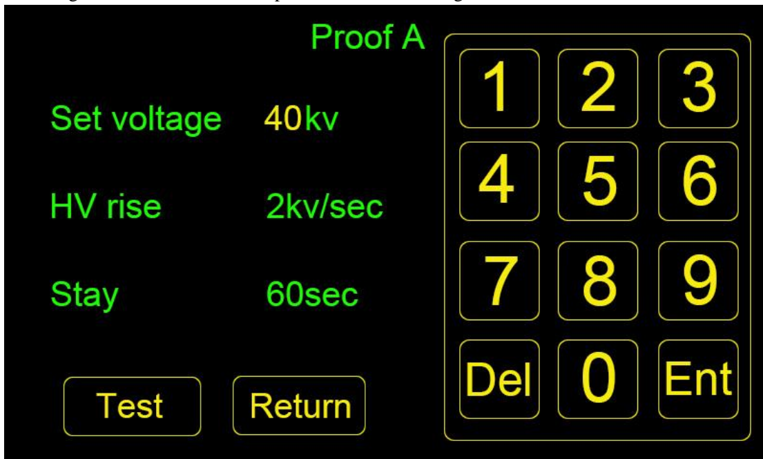
Figure 13 Proof A test set up
