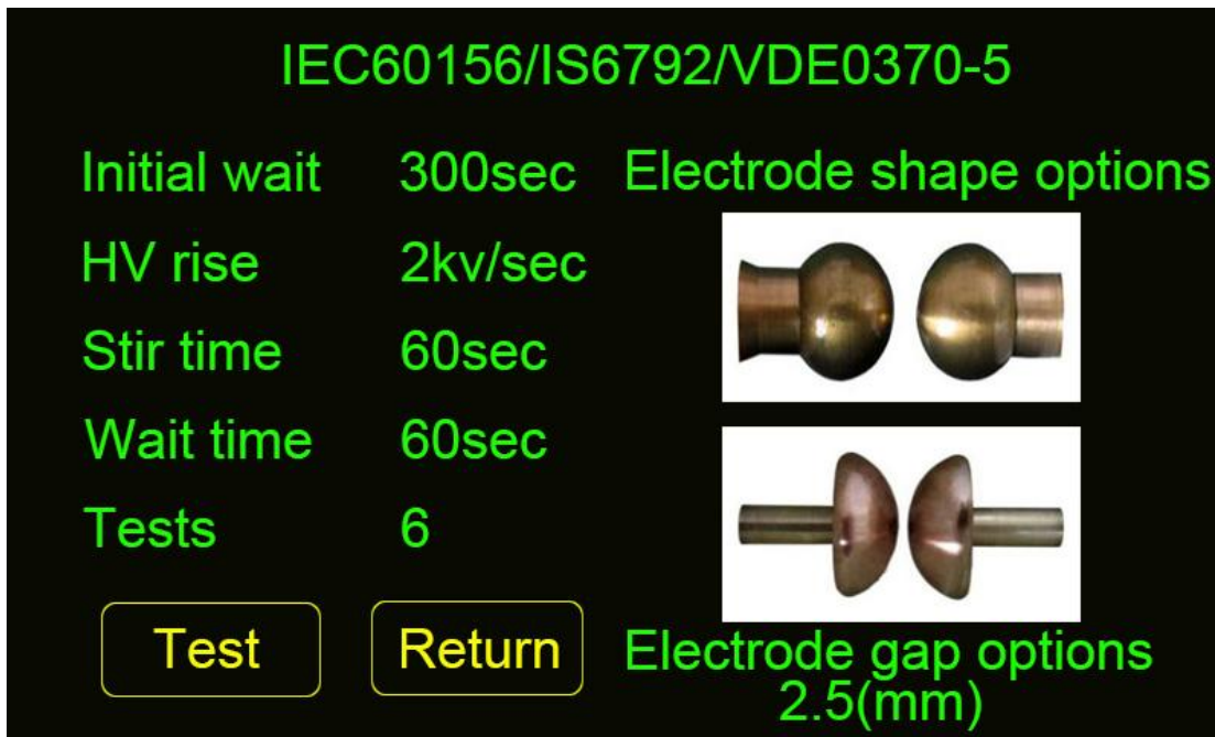
Figure 4 Parameters setting of IEC156/IS6792/BS5874
