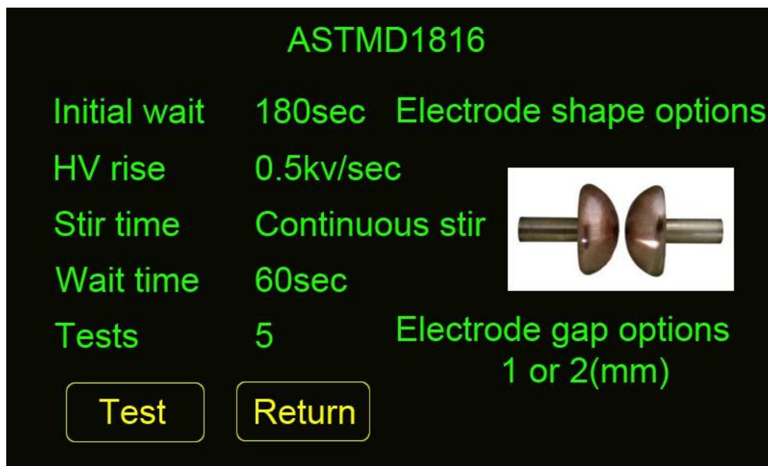
Figure 11 Parameters setting of ASTMD1816
